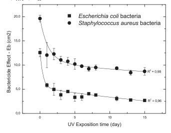
**Figure 7.**Dependence of the BWPC bactericide effect on the UV exposure time periods. BWPC produced with 2.00 wt% triclosan compound.
